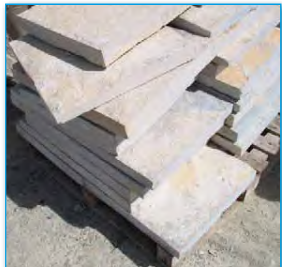
Newly prepared Purbeck stone paving
