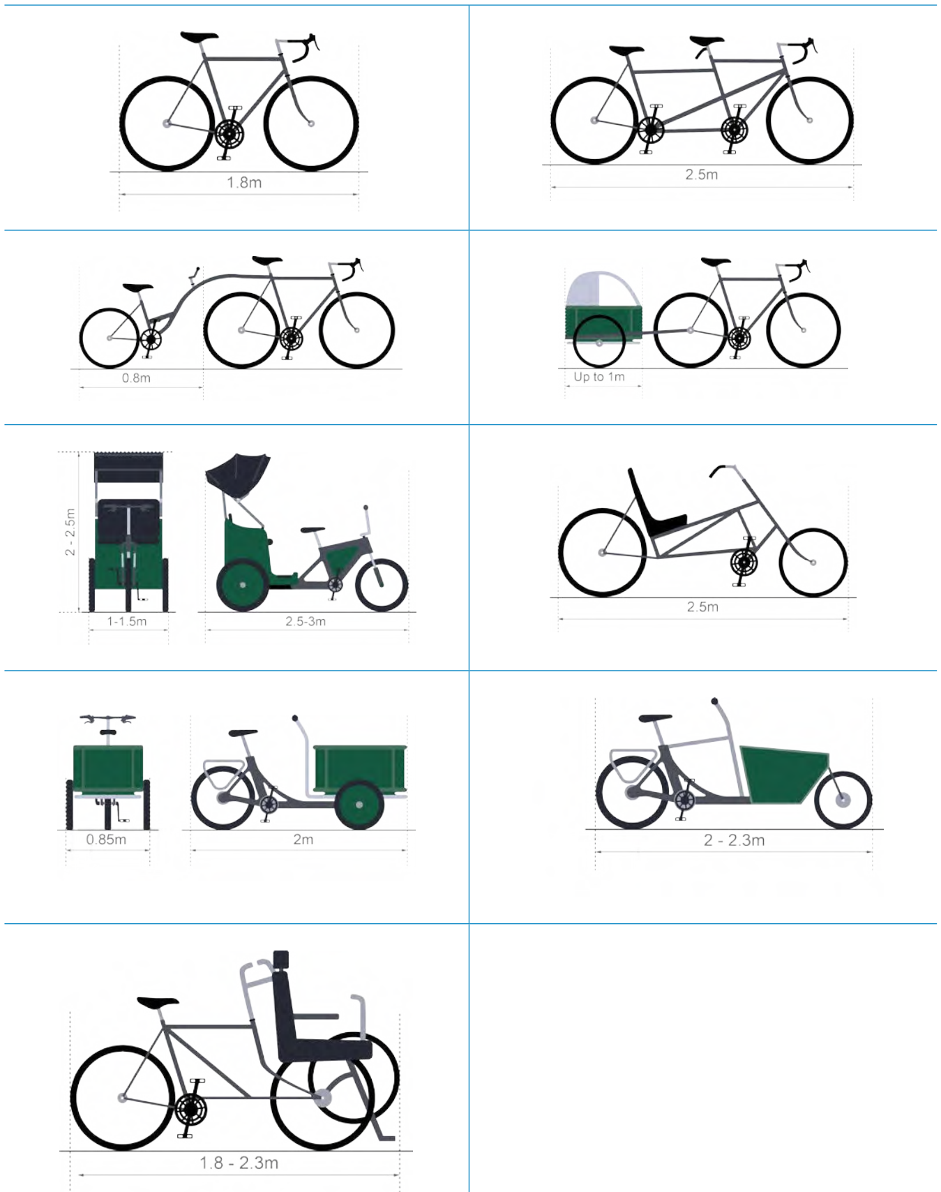
Figure 5.2: Typical dimensions of cycles
