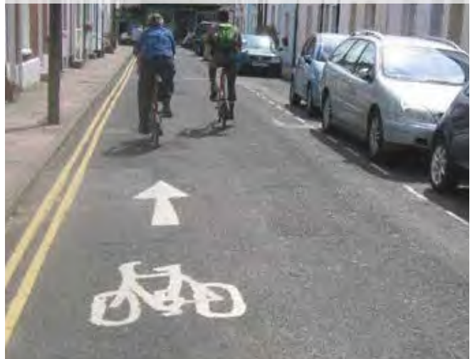
Figure 7.4: Contraflow cycling in a narrow street with no marked lane, Brighton
