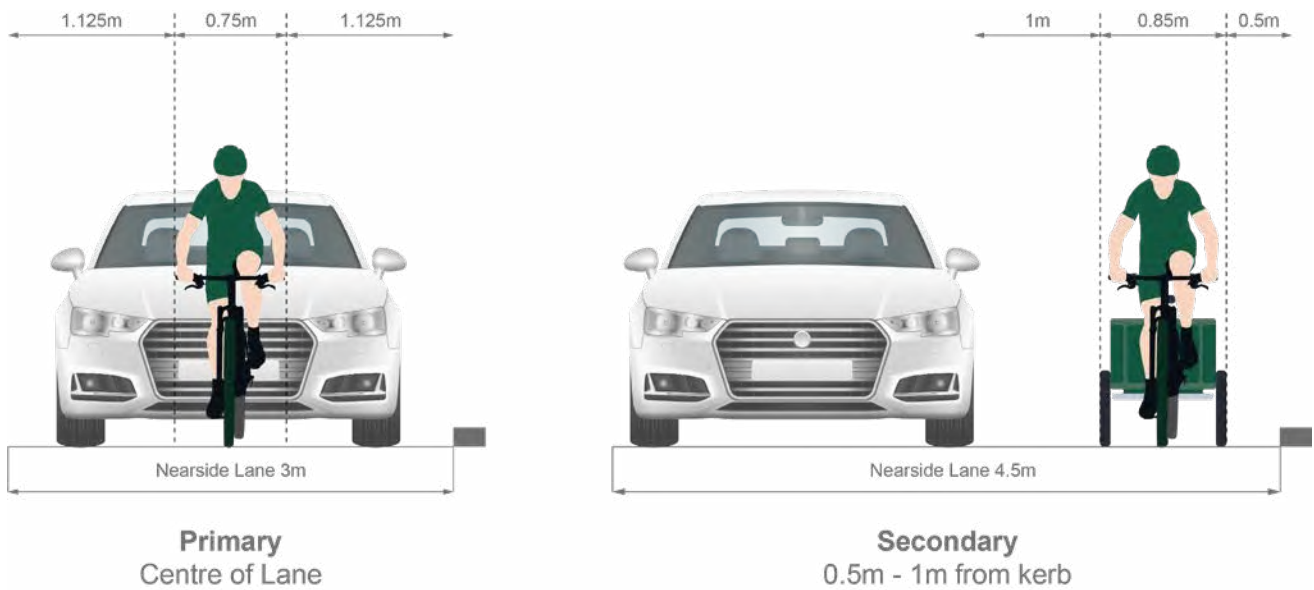
Figure 7.2: Primary and secondary riding positions
