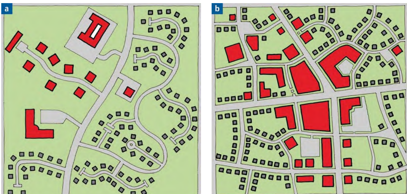
Figure 6.1: In typical post-WW2 developments (a), the main roads are often the only through routes. In more historic areas (b), there may be quiet parallel routes that could be made suitable for cycling (images from Manual for Streets)
