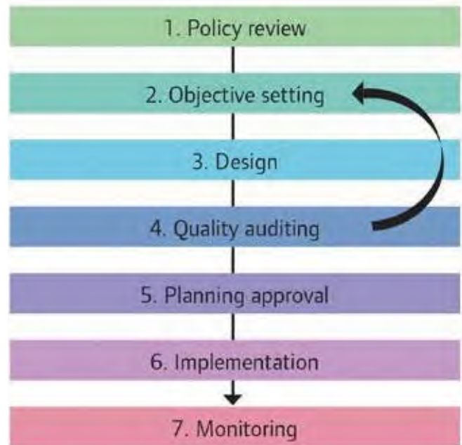
Figure 14.9: Highways, overall improvements process
