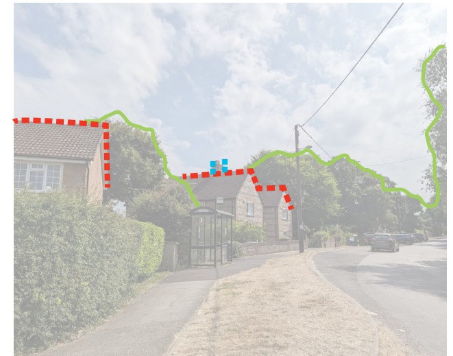
Figure 131: Local examples of roof types and rooflines in West Knighton. Elements such as vegetation (light green line), ridges (red line) chimneys (blue line), dormers (dark green line) and variations in ridges create variety and interest in the roofline.
