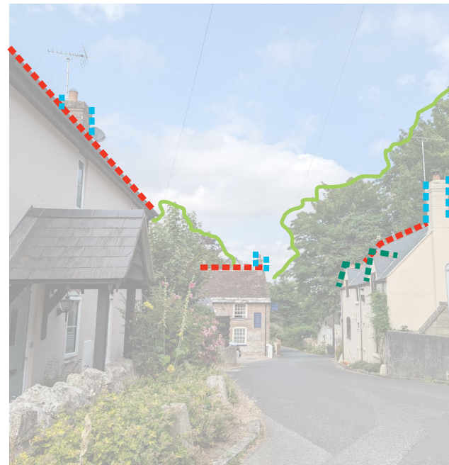
Figure 131: Local examples of roof types and rooflines in West Knighton. Elements such as vegetation (light green line), ridges (red line) chimneys (blue line), dormers (dark green line) and variations in ridges create variety and interest in the roofline.
