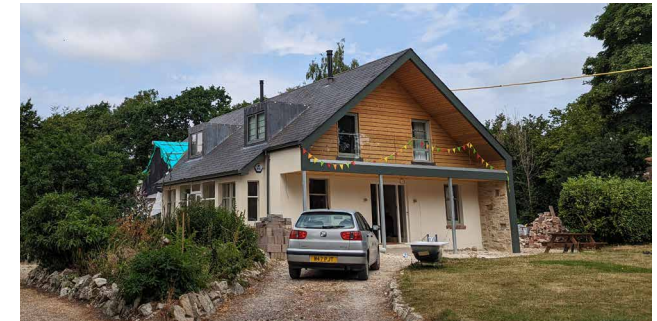
Figure 37: Local example of an eco-house with grey slate roof, off-white rendered facade and stone and orange coloured timber detailing.
