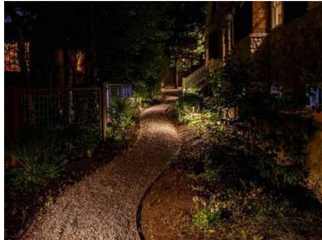
Figure 80: Example of path lighting where all lights are directed downwards, while the light sources are obscured.
