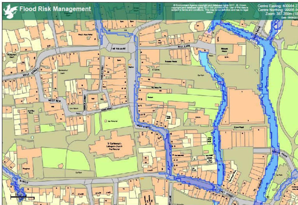
Figure 4 – Surface Water Flood Risk Areas for the 1 in 30 year and the 1 in 100 year events.
